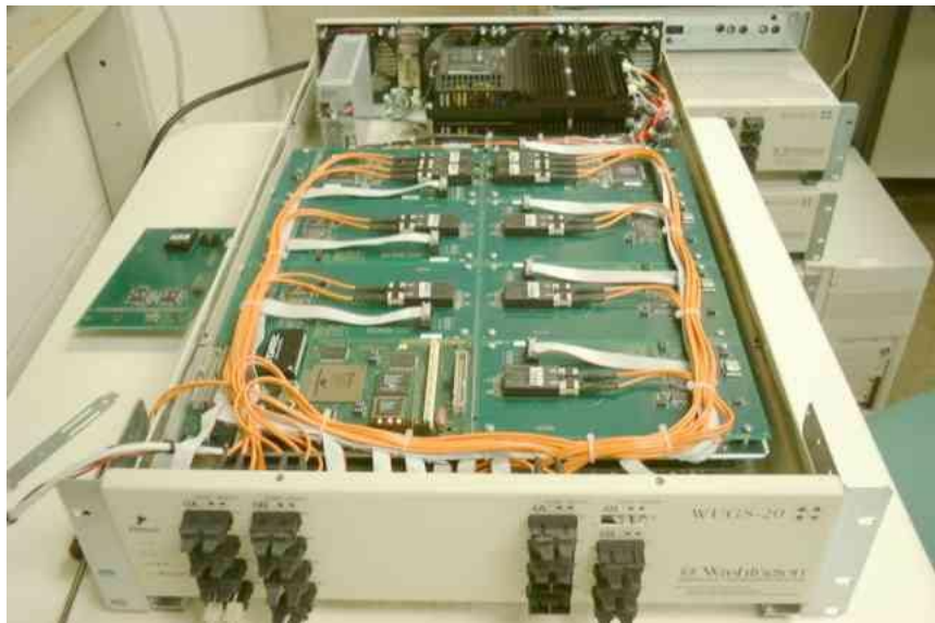
Figure 10. Photo of FPX mounted in WUGS Switch
