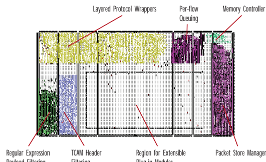
Figure 3: FPGA Layout of the SOC Firewall on a Xilinx Virtex 2000E device. Amplify software was used to constrain the areas of each of the sub-components.
