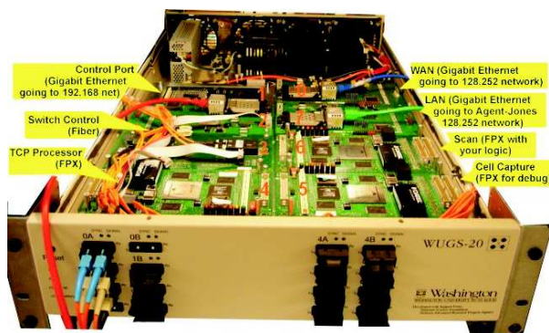
Figure 2. Photograph of the Network Processing Platform: A Washington University Gigabit Switch, three Field-Programmable Port Extender (FPX) platforms, and three Gigabit Ethernet network interfaces
